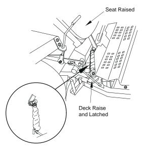
Figure 4-16 Spring Removal
